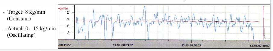
Random curve at TKS: Mg-Output from a dispenser in Co-Injection with CaC<sub>2</sub>
